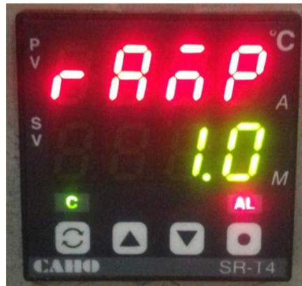
**Note:** The controller is set up to show the ramp rate (rAnP) in Deg C/min.
